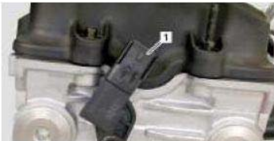
Camshaft Sensor in Cylinder Head
